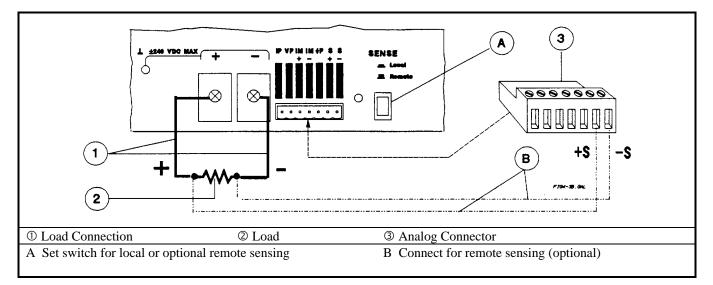
Figure 4-3b. Series 664xA and 665xA Single Load Connection
